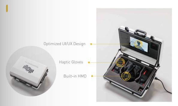
Conventional robot control interfaces are bulky, non-mobile and requires long setup time. At Telexistence Inc, we want to provide freedom and best mobility experience to our valued customers by introducing a carry on luggage type compact all-in-one cockpit package with built-in HMD, body trackers, data gloves and haptic devices. TX cockpit is airplane-approved carry-on size and weight so that our customers can access their remote robots from anywhere in the world.
